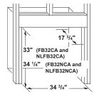
Figure 21 - Rough Opening for Installing in Wall
